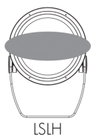
LSLH - Linear spread lens horizontal distribution
